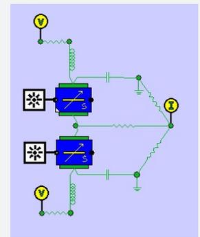
Balanced photo-detector with LRC circuit
