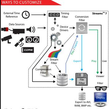
The Streams<sup>™</sup> 7 SDK allows programmers to create any of the drivers or filters shown here, or design the Streams<sup>™</sup> 7 recording engine into existing software applications.
