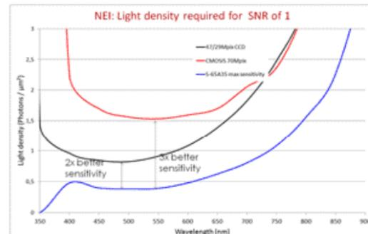
The S65 has a higher sensitivity, higher Quantum Efficiency, which allows for shorter exposure times when inspecting dark screens.
